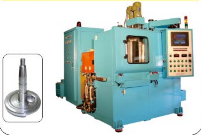
1. 50KW 高週波加熱機 50KW high frequency heating machine
