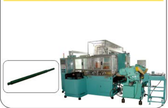
6. 臥式高週波淬火機 Horizontal high frequency quenching machine
